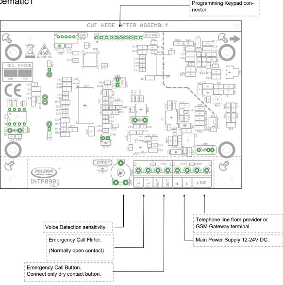
When there is an Internet line connected, a filter ADSL should be placed in the terminal "LINE".
